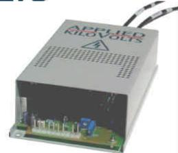
These power supplies, based on the standard HP series (data sheet HP Series refers) are intended to power imaging detectors. They give 0 to +3.5 kV and can be floated on voltages up to ±2.5 kV (HFxx2.5), ±10 kV (HFxx010), ±20 kV (HFxx020) & ±30 kV (HFxx030) and use differential feedback techniques to allow the **24 volt power, control** and **monitor** signals to be at **ground potential**.
